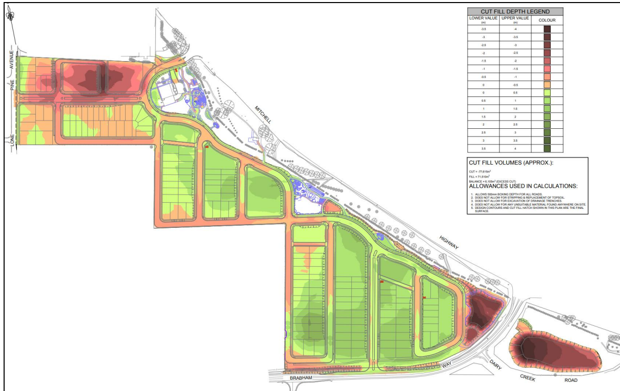
Figure 7 - bulk earthworks (red = cut, green = fill)
